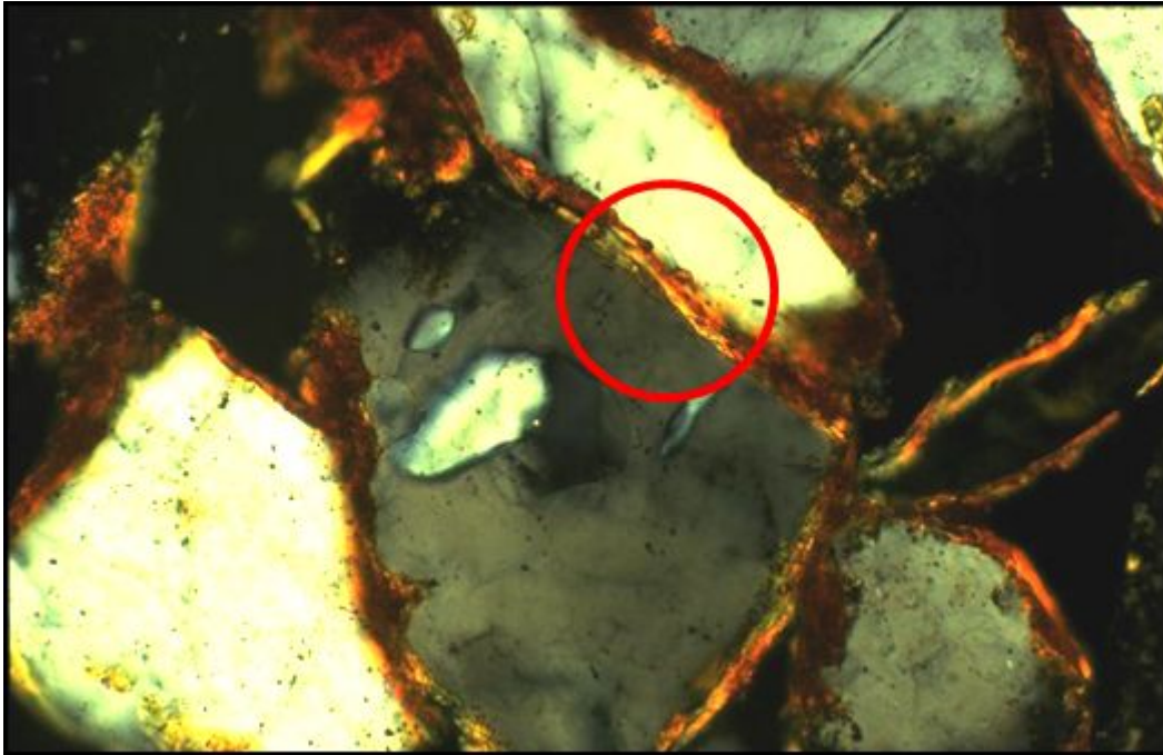
Photo 1: Iron coatings on the outside of sand grains (Photo: G. Peek, WUR)
